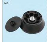
Rotor Capacity: 100mlx8 Max Speed: 12000r/min Max RCF: 19830xg Adapters: 10ml, 20ml It is customizable
